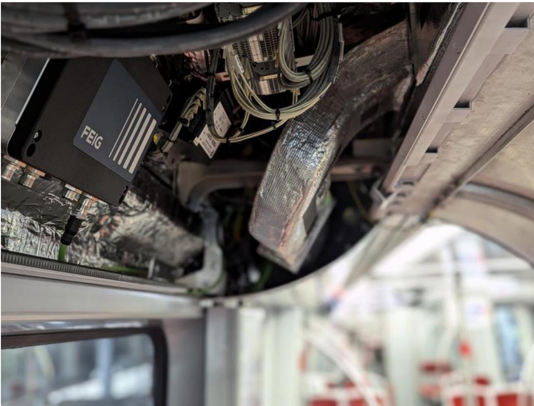
FEIG RFID reader ID LRU4000X installed in the vehicle (source: FEIG)
