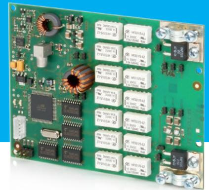
The Dynamic Antenna Tuner ID DAT is designed for automatic tuning and retuning of RFID Long Range Antennas with an operating frequency of 13.56 MHz. The parameters for setting the antenna are measured on the board under operating conditions. The antenna tuner is also able to disconnect the antenna circuit through an electronic switch up to a certain power.
