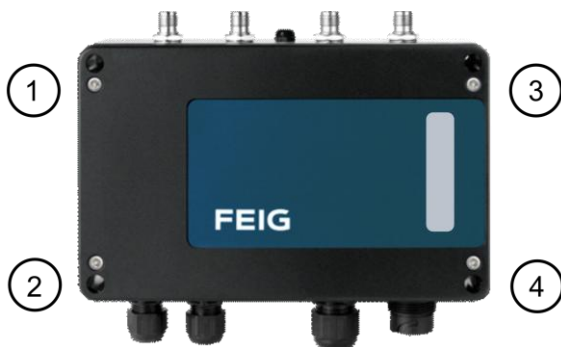
Fig 7: Open the screws of the housing cover
